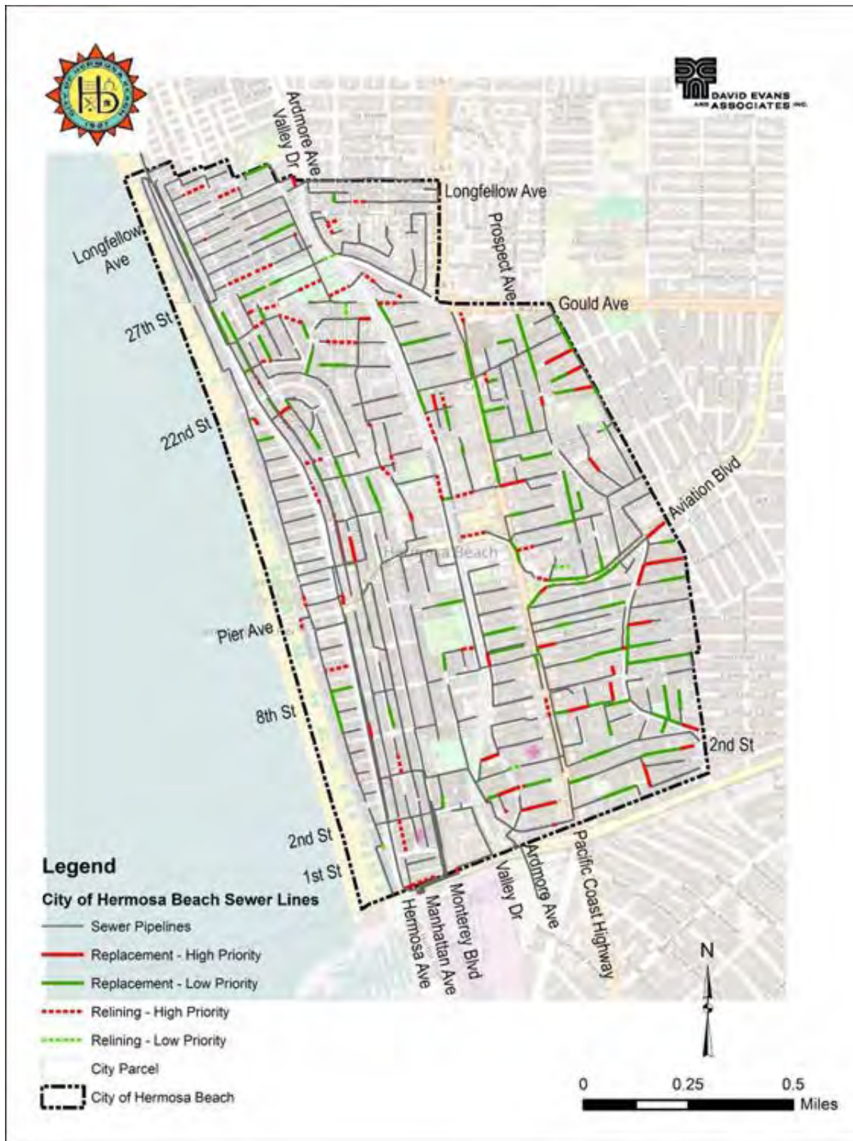
Figure 5-3: Sewer System Defects Recommended for Rehabilitation
