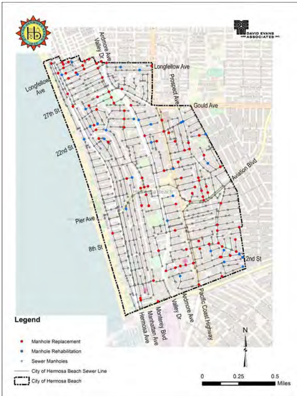
Figure 5-6: Manholes Recommended for Improvements
