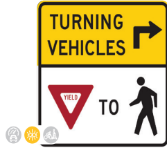
Yield Signage Increases driver awareness of the presence of bicyclists and pedestrians.
