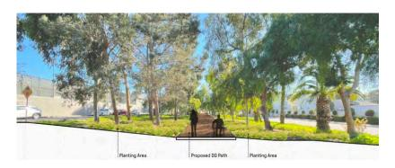
This project will remove woodchips and construct an accessible pedestrian trail composed of decomposed granite on the Greenbelt between Pier Avenue and 8th Street.
